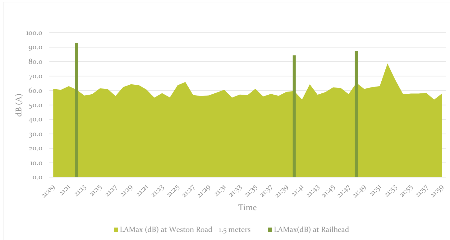
Figure 7-15 Measured L_{A\text{Max}} at Weston Road at 1.5m with Three Highest Railhead L_{A\text{Max}} Noise Events Shown
